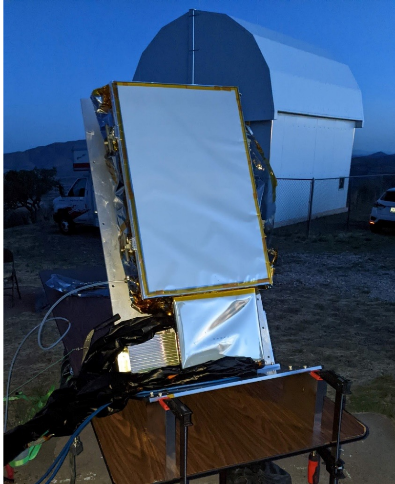
EM WFI During Starfield Testing @ McDonald Observatory (Analysis Underway)
