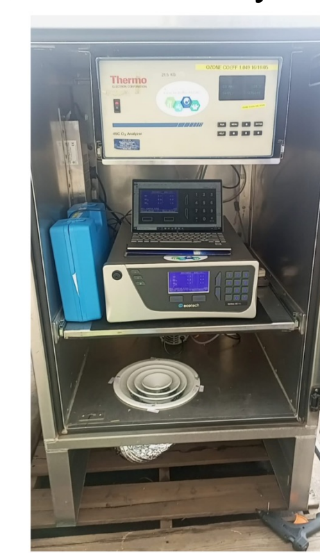
Figure 8: NO x monitoring with chemiluminescence NO x analyzer in CBD, Nairobi, Kenya
