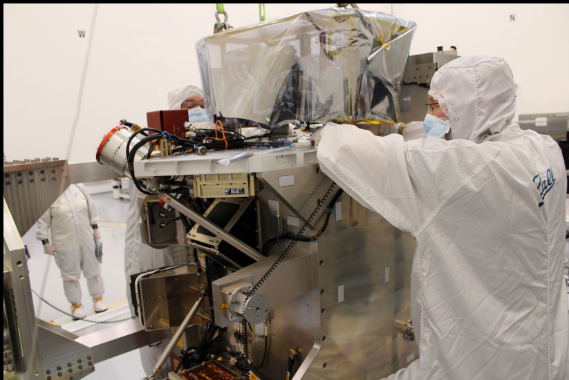
Compact Coronagraph (CCOR) installation on SWFO-L1
