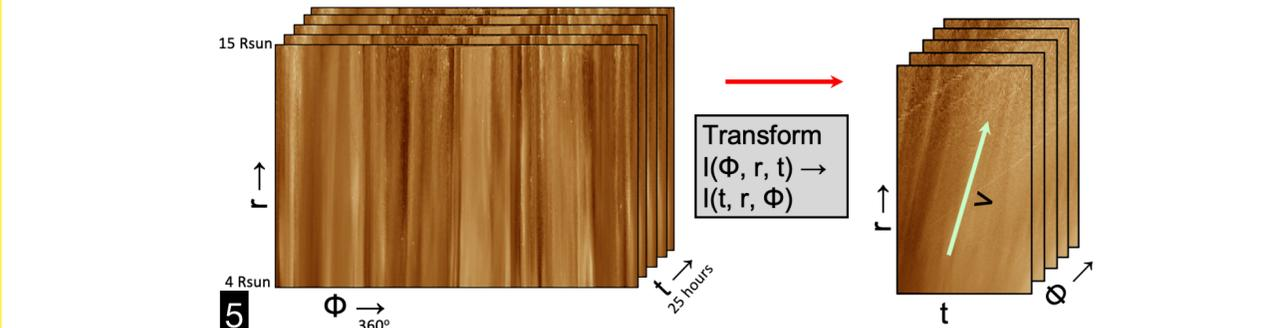
**Fig 5.** The collection of images at different times allows us to transform the image coordinates from spatial-spatial  $(\phi, r)$  to spatial-temporal  $(t, r)$ . (Source: [2])
