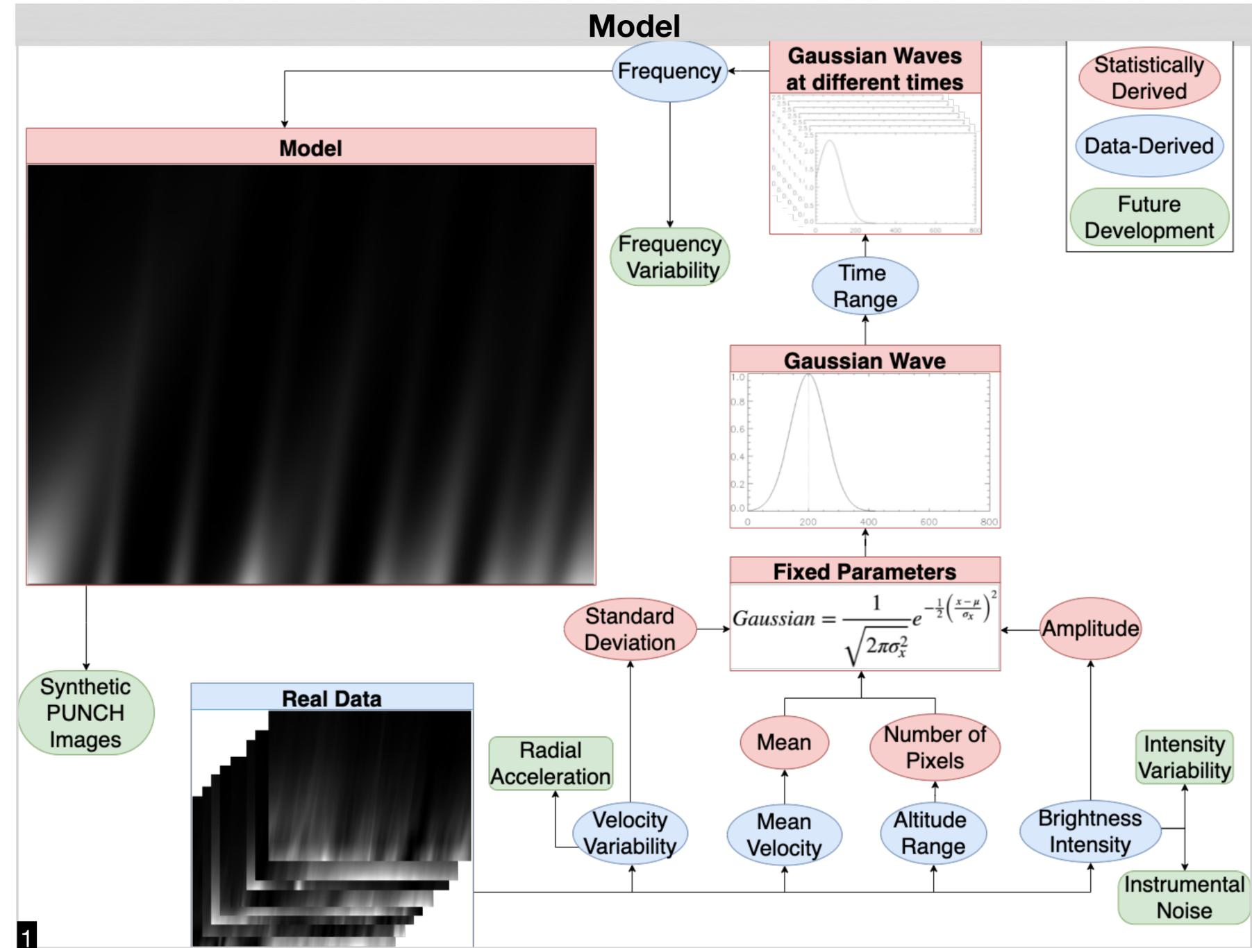
**Fig 1.** Flowchart of process to create a synthetic corona outflow. In blue, fixed parameters used in our model come from previous observations, such as STEREO-A / COR 2. In red, each parameter controls one aspect of the Gaussian wave, in particular its central position, width and height. In green, features still in development for our model. Our model can easily be extrapolated to altitude ranges of future mission like PUNCH.
