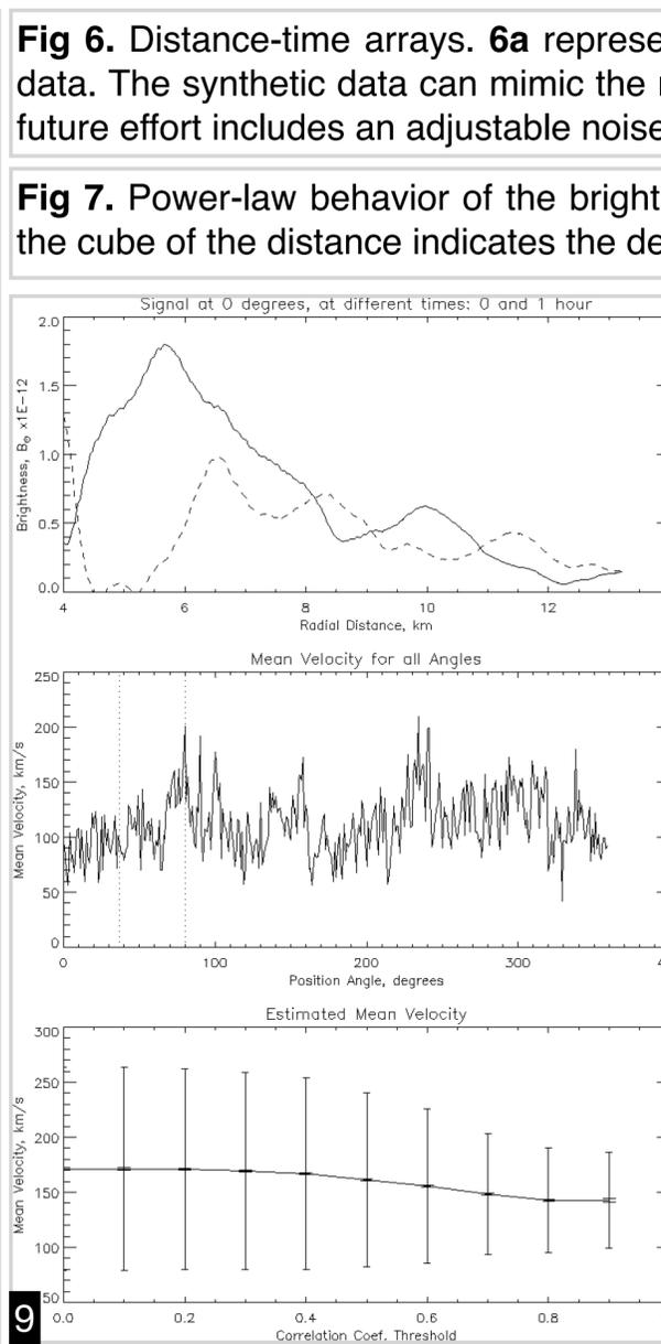
**Fig 9.** Velocity exploration. The estimated velocity was obtained using a cross-correlation technique. This velocity could be assessed by any other flow tracking algorithm.
