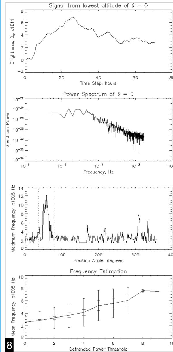
**Fig 8.** Frequency exploration. The estimated frequency was taken by accounting the maximum frequency for each position angle. This frequency can gauge the amount of features a certain position-time array exhibits.
