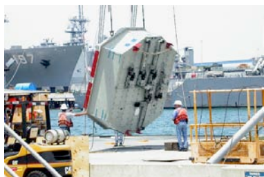
SPY-1 S-Band System – Antenna being removed from a ship. These systems or subsystems are available to DOD through a transfer process.
