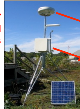
Off-the-Grid Radar First node being tested at UMass
