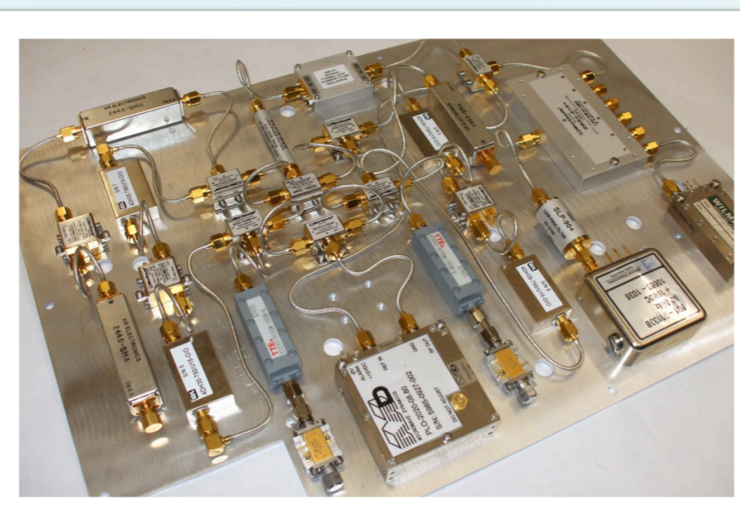
Each up-down-conversion unit is housed in a custom-made 1U enclosure (0.75").
