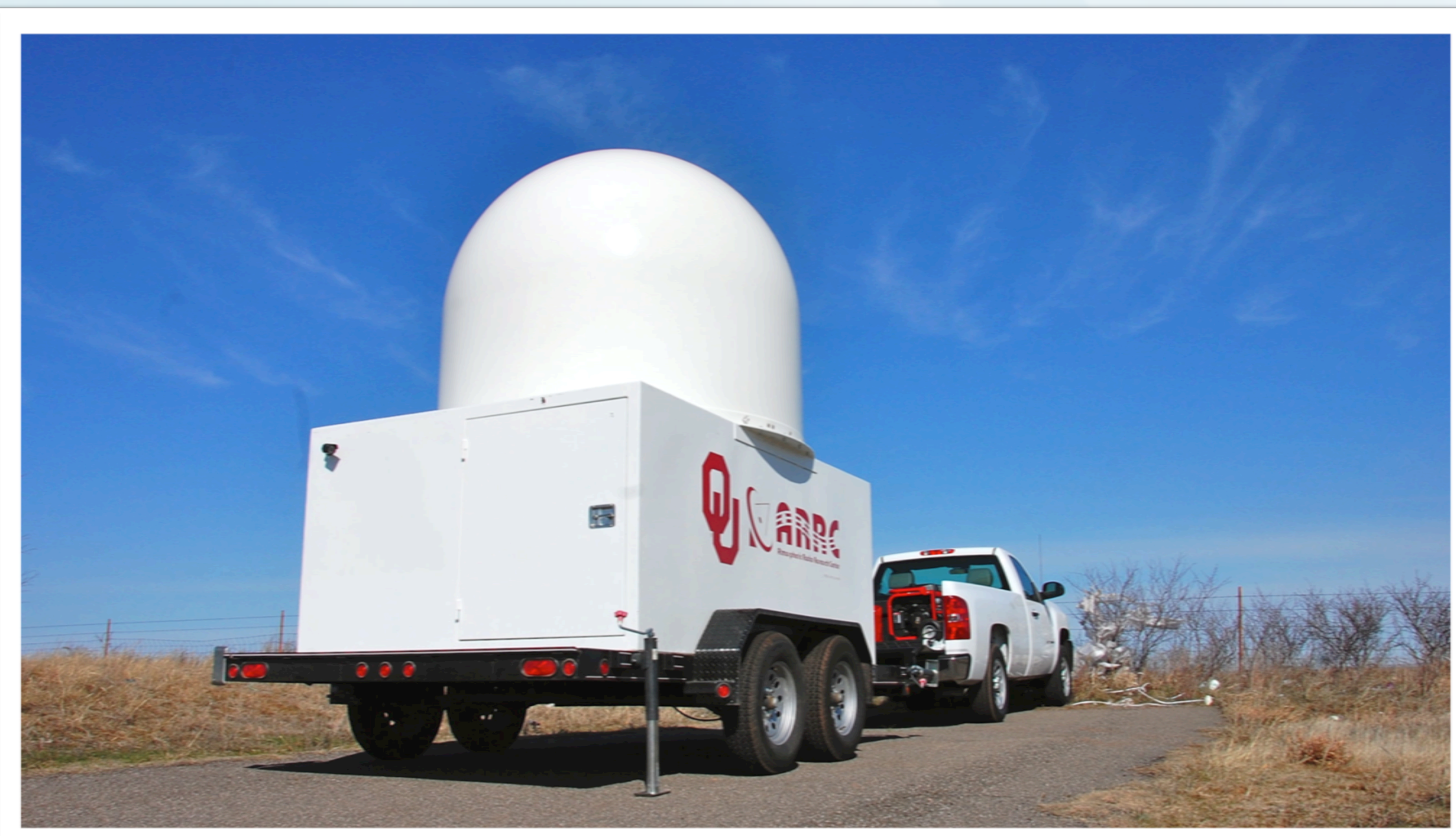
The PX-1000 radar in the field. The entire trailer with the radar system weighs approximately 4,500 lbs., which can be easily towed by a full-size pickup truck.
