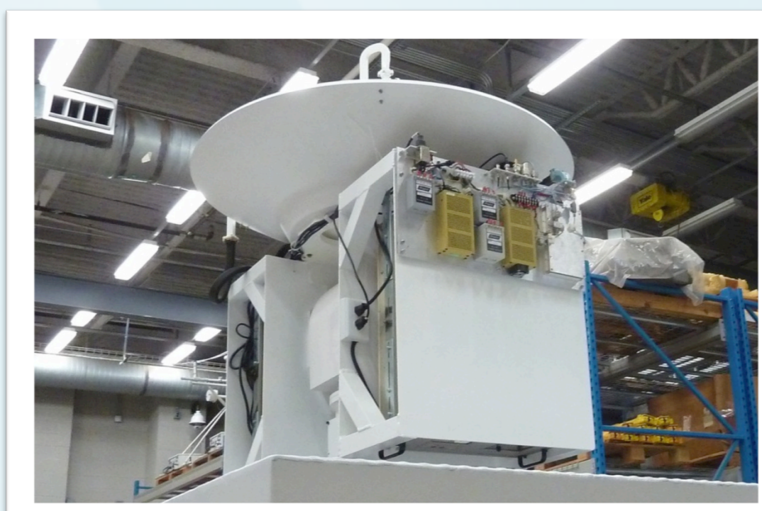
Frames on the side support all the RF components, i.e., IF transceiver, up-down-conversion units and amplifiers
