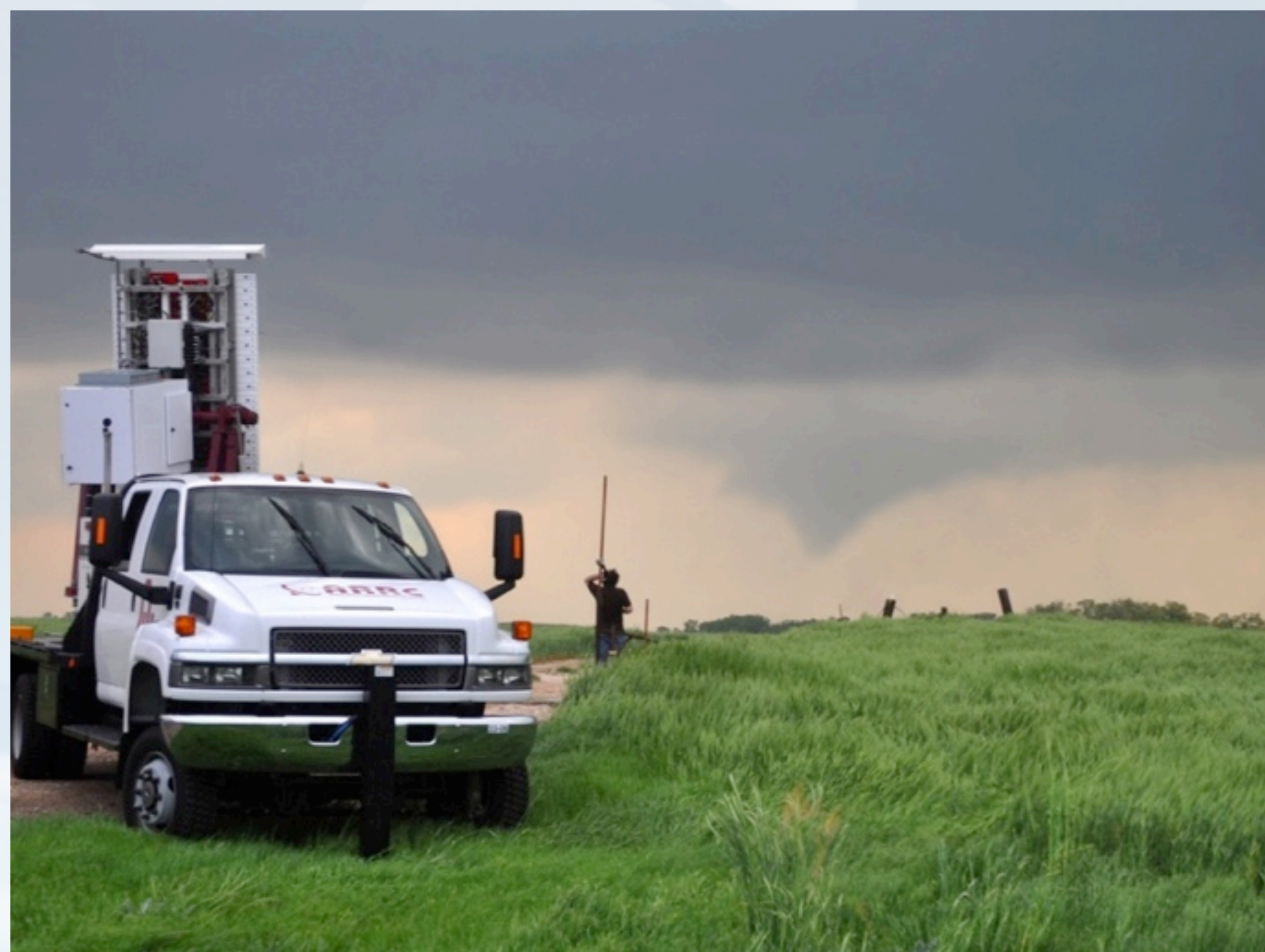
The AIR deployed to observe a tornado near Carmen, OK on April 14, 2012. These are the first simultaneous cross-section measurements through a tornado.
