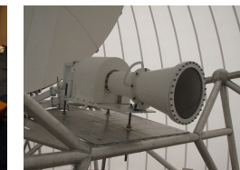
10-cm (S-band) Feed Assembly
