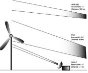
•The clear air deployment resulted in patterns consistent with beam blockage and multipath scattering.
