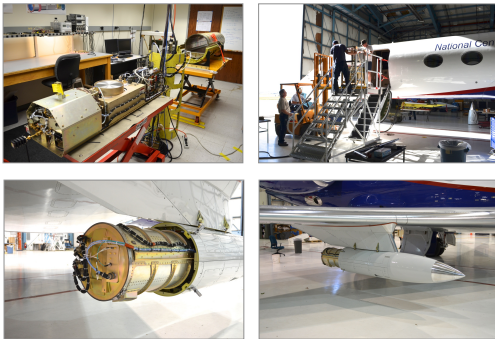
HCR installation and GV integration (clockwise from top left): Bench-top Installation, aircraft upload, EMI test on the wing and pod mechanical fitting.
