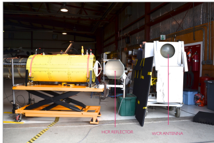
WCR and HCR inter-comparison setup.
