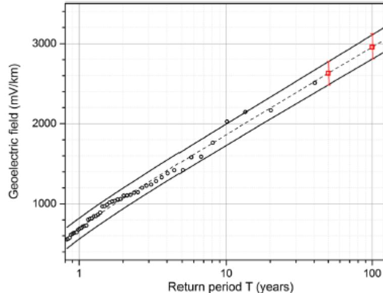
Fitting of the peak geoelectric fields (circles) in Victoria and Ottawa to an extreme value distribution (dashed line) with 99% confidence intervals (solid lines). The predicted values once per 50 years and once per 100 years are denoted by red squares.
