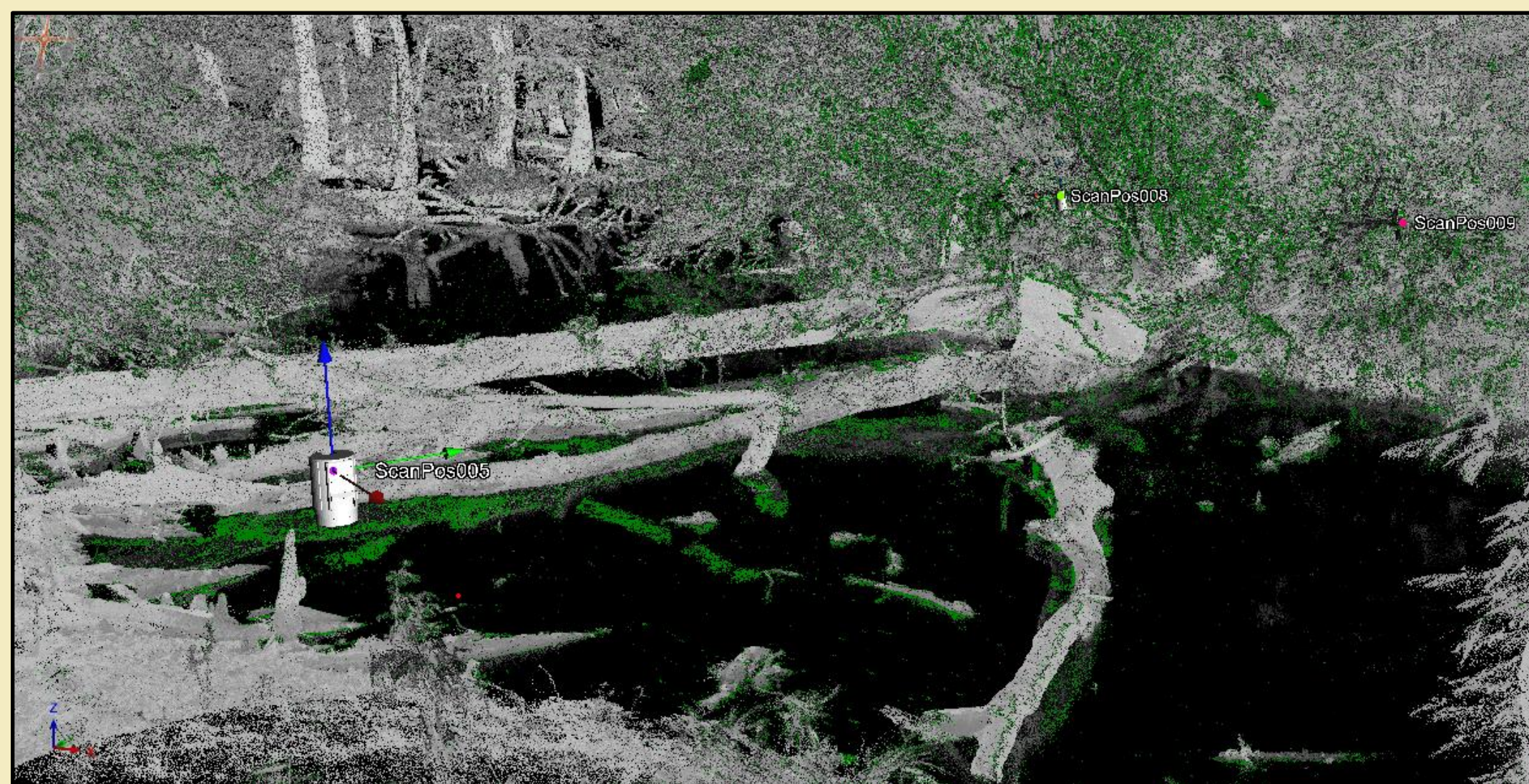
Figure 4. 3D point cloud generated from terrestrial LiDAR scans of Chokey Creek (CHO)
