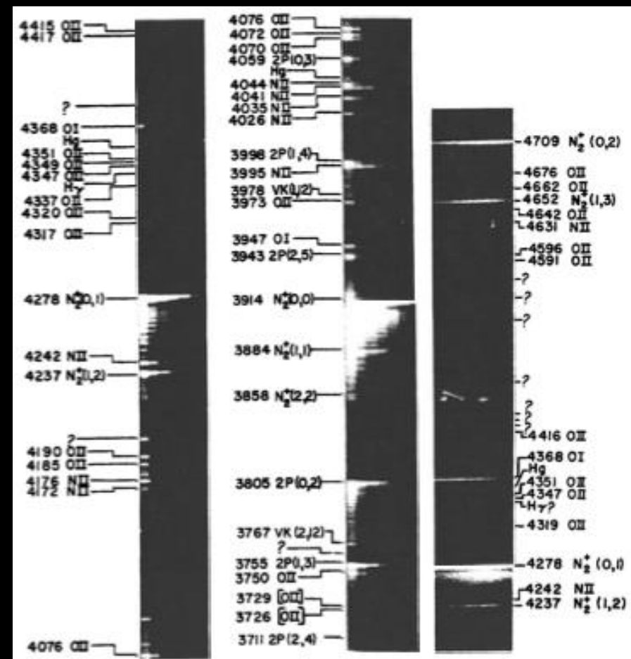
FIG. 5.3. Auroral spectra, 3700-4750 Å. The spectrum 3700-4430 Å was obtained with a dispersion of 22 Å/mm during the great red aurora, 11 February 1958. The one on the right is from an ordinary green aurora, 10 November 1956; dispersion 33 Å/mm. From Yerkes Observatory plates nos. 128 and 77. Tracings are shown in Figs. 5.11, 5.12, and 5.13.
