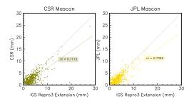
The scattergrams visualize the correlation of the amplitude of the annual signals for all of the GNSS stations included in JTRF (roughly 530) and estimated on the GGFO-derived elastic displacements and the GNSS observations. The m values reported in the plots represent the correlation between the two data types.
