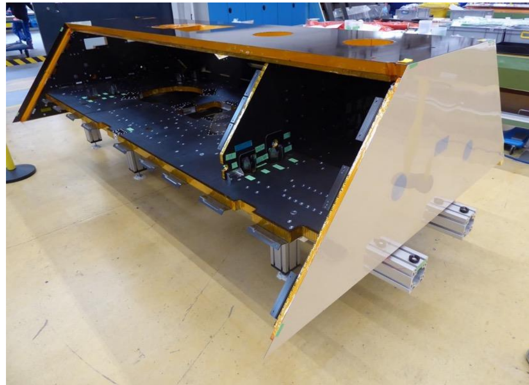
FM1 Solar Array fit check
