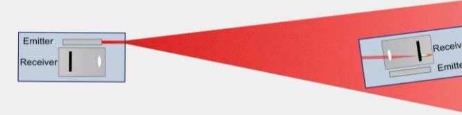
**MiniCAS:** compact optical system enabling instantaneous attitude acquisition with microradian sensitivity
