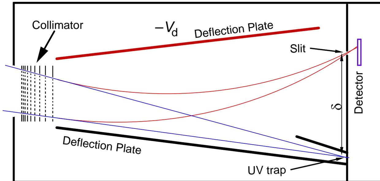
The main advantage of a SADA is that particles up to several MeV/charge can be deflected since  $K$  can be large and large deflection voltages can be supported
