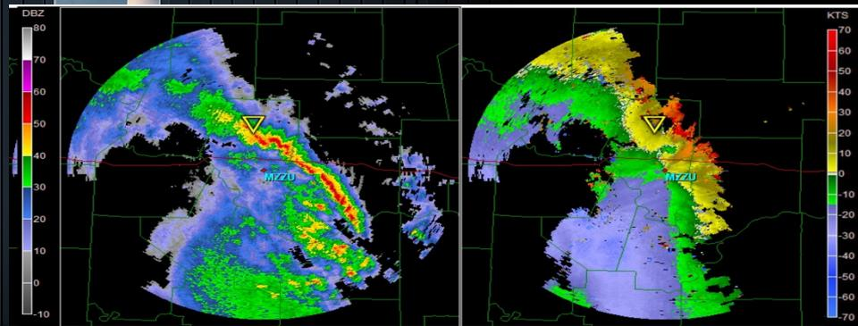
Sample of MZZU Research Radar data detecting a confirmed small tornado through identifying low-level wind rotation.
