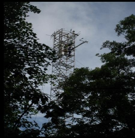
The Eddy covariance (EC) systems measure horizontal and vertical wind, air temperature, and fluxes of carbon dioxide, water vapor, and sensible heat. Solar, longwave and photosynthetically active radiation are also measured. EC systems are also in agricultural lands north of the Missouri Ozarks AmeriFlux site (Oak-Hickory forest) to determine the eclipse effects over multiple ecosystems.
