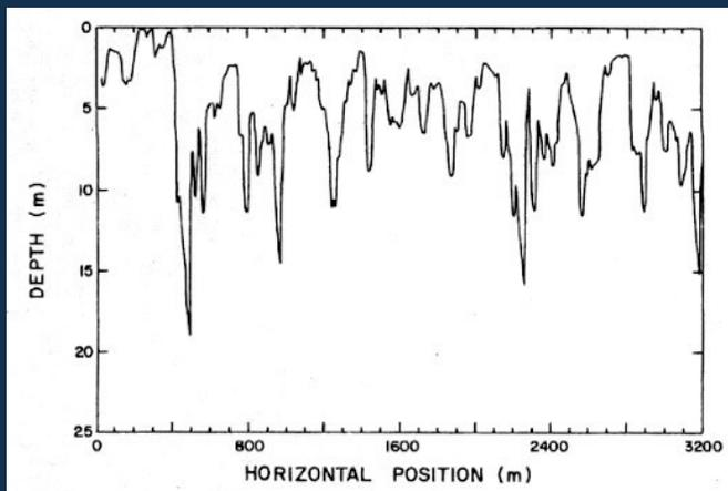
A submarine sounding of sea ice draft in the Arctic (Thorndike et al., 1975)
