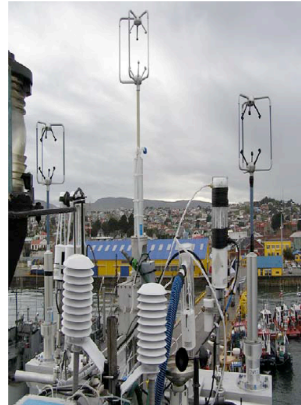
Figure 1. Cluster of sonic anemometers, fast humidity sensors, and mean T/RH sensors on the jackstaff of the NOAA Ship Ronald H. Brown for GASEX-3. The PSD sonic is in the center. The sleeved fast-sample LI-7500 is the unit on the right with the large blue ventilation tube. The two open path units are on the left. Each sonic is mounted to its own motion-measuring system.
