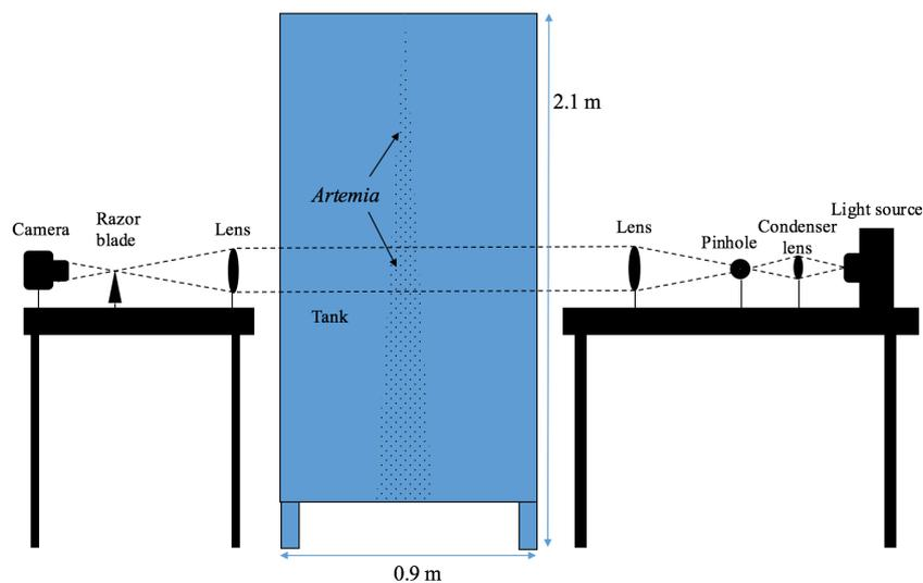
Figure 5: Schlieren imaging system described in section 2.2.
