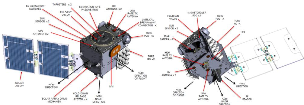
SC Deployed Configuration
