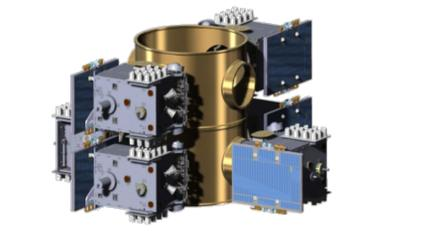
Stowed Launch configuration on the launcher
