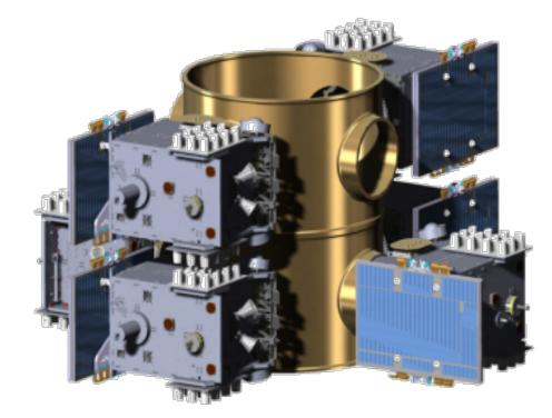
Stowed Launch configuration on the launcher
