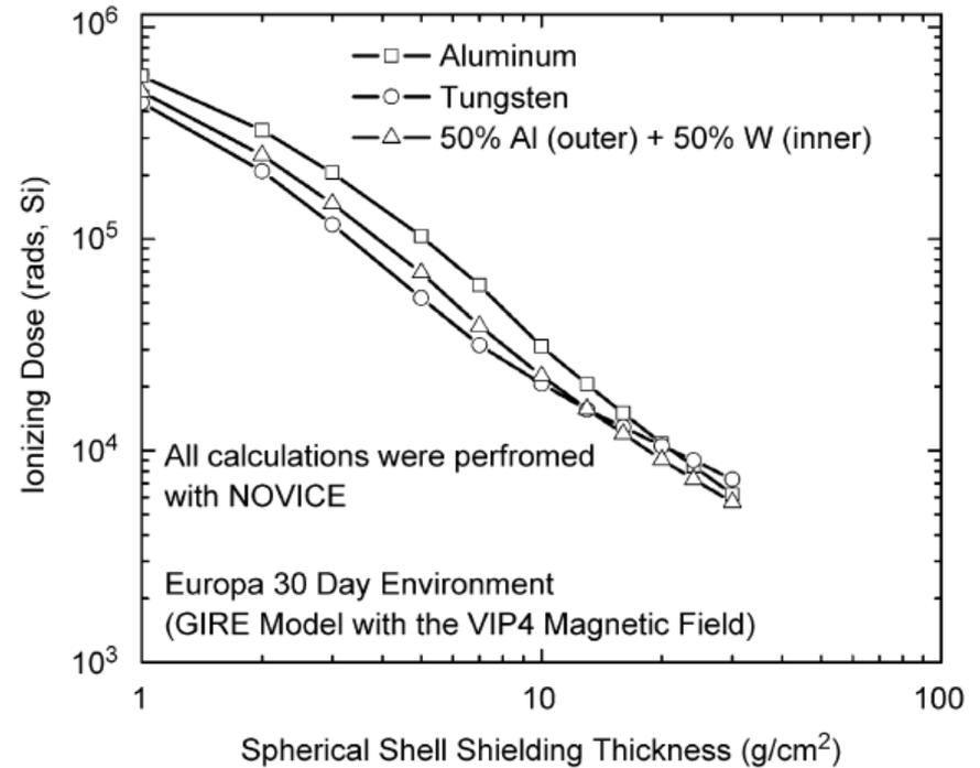
Fig. 3. Ionizing doses calculated with NOVICE for a detector located at the center of the spherical shell shielding of aluminum, tungsten, and 50% areal mass aluminum (outer layer)/50% areal mass tungsten (inner layer) combination in a 30-day Europa mission. (100 rad = 1 Gray).
