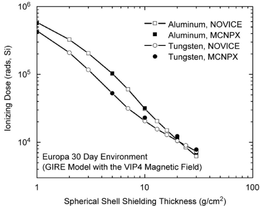
Fig. 2. Ionizing doses calculated for a detector located at the center of spherical shell shielding of aluminum and tungsten in a 30-day Europa mission with NOVICE and MCNPX, respectively. (100 rad = 1 Gray).
