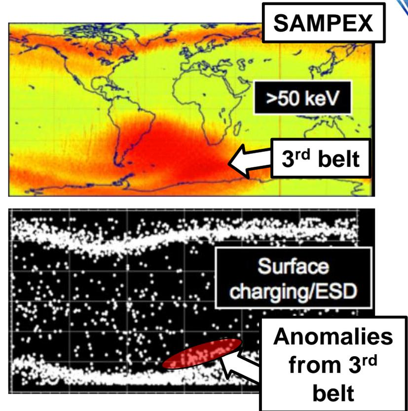
***Third (or fourth, or more) new electron belts won't drive satellite designs via total dose or vehicle charging unless the orbit is circular, equatorial, and stays near L=2.***
