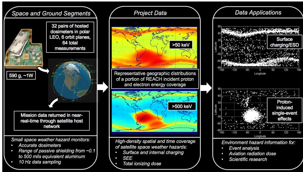
Figure 1. REACH operational view. The space segment consists of hosted pairs of dosimeters whose data flow through the in-space satellite network for ground processing. The project data are dose rates sampled from 32 separate satellites with a wide range of equivalent shielding for engineering and scientific applications. Environment and spacecraft effects examples are from the SAMPEX mission.
