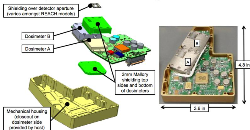
Figure 2. Expanded view of the primary REACH pod components: mechanical housing; single printed circuit board with interface circuits and circuitry for buffering and packetizing of telemetry; dosimeter detectors and their shielding. The photo on the right shows the pre-integration configuration of a Model 3 pod with outer dimensions. The labels A and B correspond to dosimeter identifications in the REACH telemetry.
