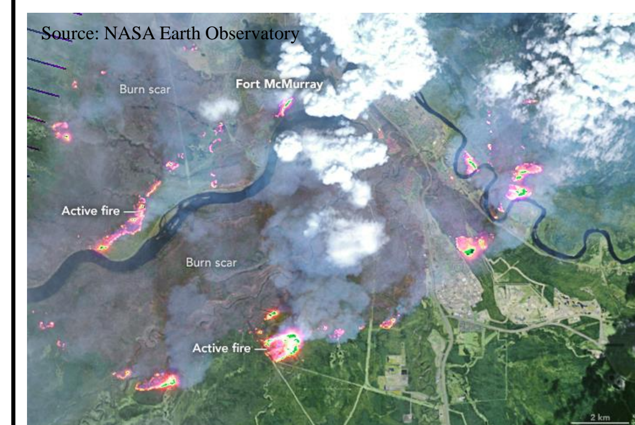
Figure 12: Infrared, near infrared and green-light images from Landsat 7, taken on May 4 th 2016 are combined here to penetrate the clouds and reveal burn scars and hot spots.
