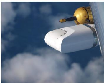
MTP fairing with high-density polyethylene window. The Ultra High Sensitivity Aerosol Spectrometer (UHSAS) is mounted next to MTP.
