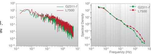
Figure 3: Spectral Density of H<sub>2</sub>O and CO<sub>2</sub>. The low frequency response of the instruments is well matched. The L7500 is high in the flux frequency response range.
