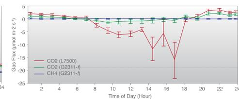
Figure 5: CO<sub>2</sub> and CH<sub>4</sub> diurnal fluxes (5 day composite). WPL correction is applied to 7500 data
