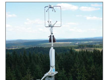
Gill 3D Sonic Anemometer Picarro Sample Inlets at 30 m Wetzstein
