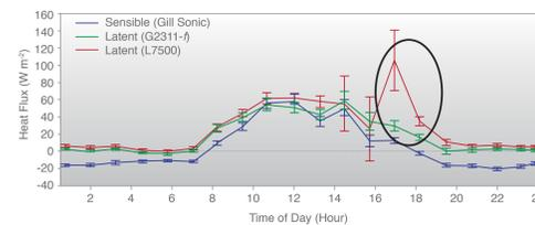
Figure 4: Latent and Sensible Heat Flux (5 day composite) There is generally good agreement between the two instruments during the observation period except for the circled excursions in the L7500 data due to liquid water accumulating on the mirrors. During this period daily temperatures ranged between 92 and 115 degrees F, which created large fluxes during the day.
