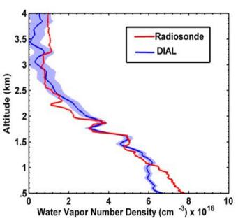
Data on the last two slides were collected with tunable external cavity diode seed lasers.
