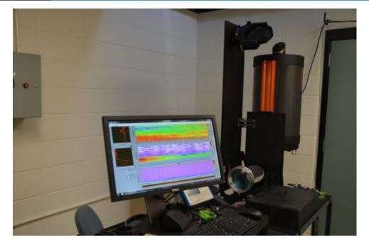
The DIAL instrument operating in the Roof-Port Lab at Montana State University.
