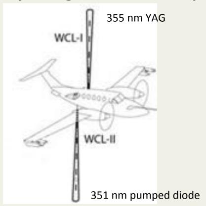
Compact polarization lidar (elastic)
