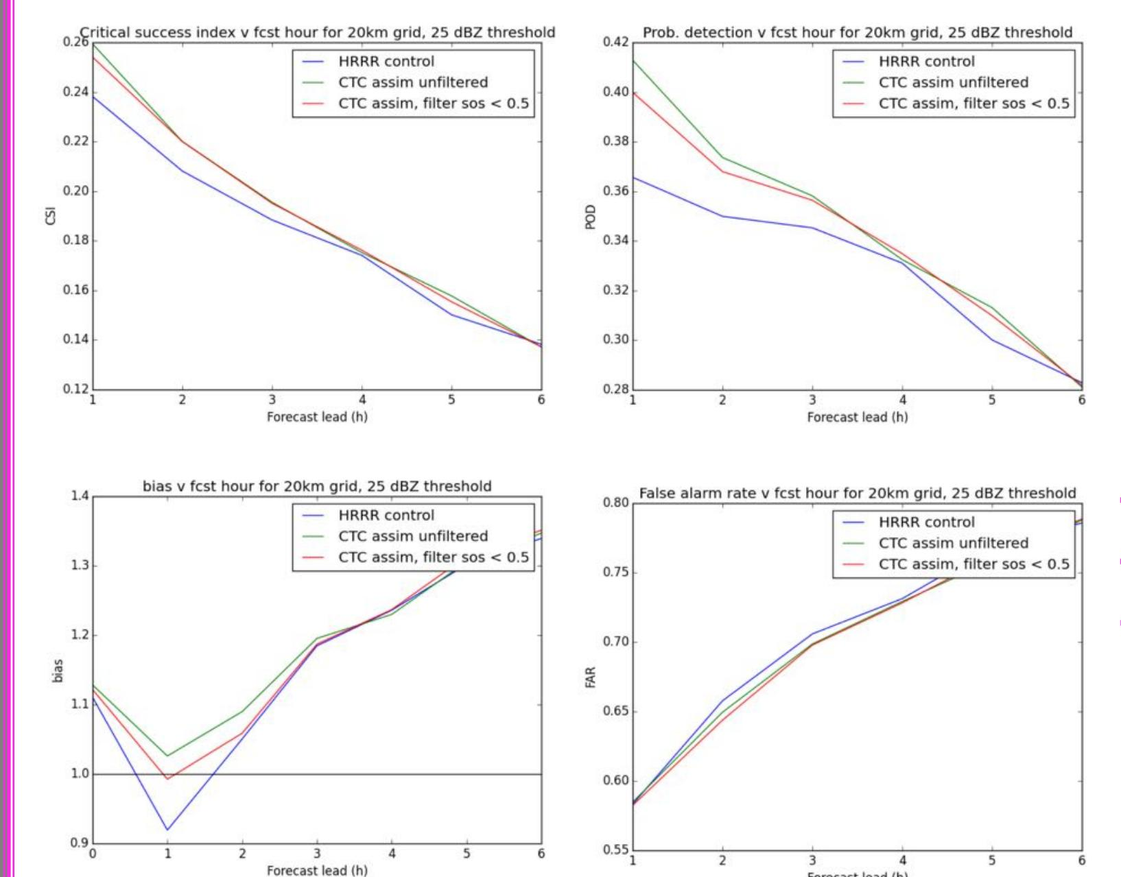
**Left: verification statistics as a function of forecast lead time, averaged over 5 hours during the test case**
