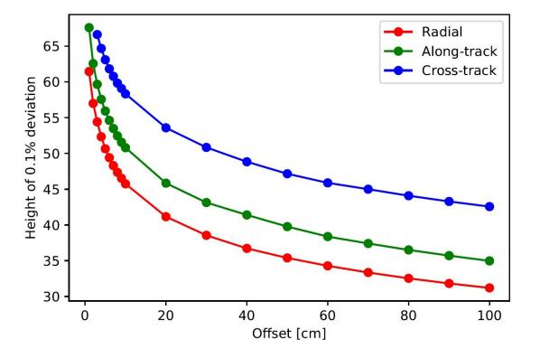
% of bending angle bias as a function of antenna phase centre offset for different heights
