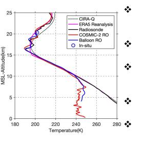
Comparison among balloon-borne RO, radiosonde, COSMIC-2 RO and ERA5 reanalysis for a typical profile. They are all within a 2-hr time interval and a 300-km distance separation. ROC2 dry temperature closely matches the radiosonde and COSMIC-2 above 10 km and resolves the tropopause very well. Similar wave pattern can be identified in all observations, but not in the reanalysis. 220 240 260 280 **C** Differences below 10 km are due to the simplified dry temperature retrieval process.
