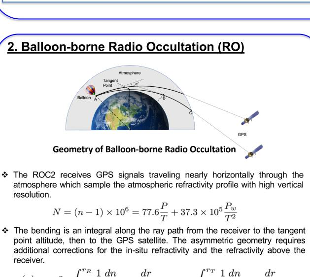
$$\alpha(a) = -2a \int_{r_t} \frac{1}{n} \frac{dn}{dr} \frac{dn}{\sqrt{n^2 r^2 - a^2}} - a \int_{r_R} \frac{1}{n} \frac{dn}{dr} \frac{dn}{\sqrt{n^2 r^2 - a^2}}$$
