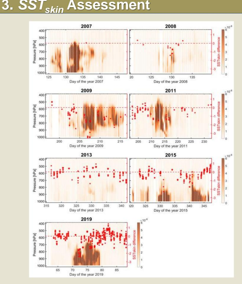
SST<sub>skin</sub> difference from each of the ship tracks. Red stars indicate the difference with the right y-axis range. The operations of M-AERIs are suspended during rain thus causing some SST<sub>skin</sub> data gaps along the track. Comparisons in and close to ports are not used. The background color indicates the dust mixing ratio.
