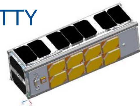
Antenna Array: 8 segments, L1, RHCP, 16 db
