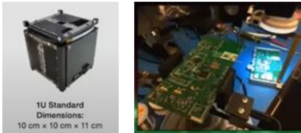
Figure: (Left) a CubeSat and (right) an example of inside circuit design in a CubeSat.
