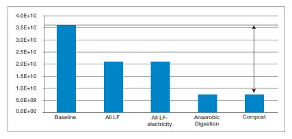
Annex Figure 4: Life-cycle GHG Emissions (CO<sub>2</sub>e/year) for all Scenarios (Anaerobic digestion and composting offer the greatest emission reductions.)
