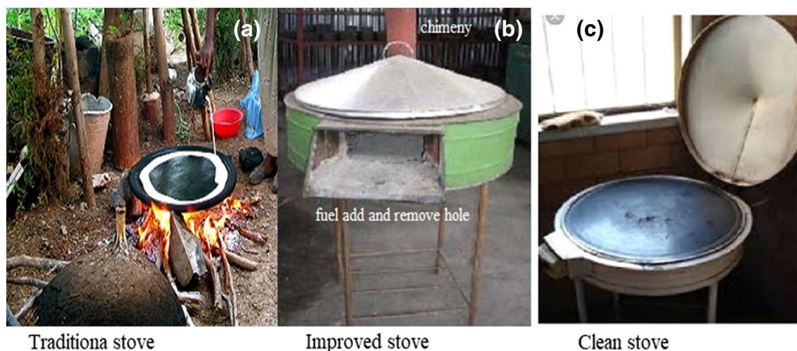
Fig. 1 The three different types of stove used for the baking of Injera . a Traditional open wood-burning stove, b improved-efficiency wood-burning stove, c high-efficiency electric stove
