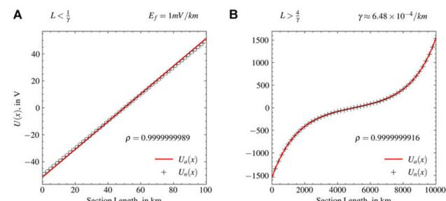
Figure 5. Distribution of voltage, estimated using theoretical approximation (red) and computational model (black "+"), along the (A) electrically-short and (B) electrically-long Ocean-Earth sections. The correlation coefficient between theoretical and numerical estimates are provided in each panel.  $L$  and  $1/\gamma$  are the physical length and adjustment distance of the cable, respectively.
