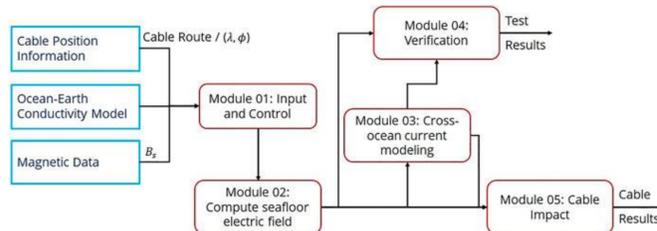
Figure 1. Control flow diagram of operations done by computational model. The boxes in red and blue define operational and input modules, respectively. Solid lines represents data flow interconnections between different modules.
