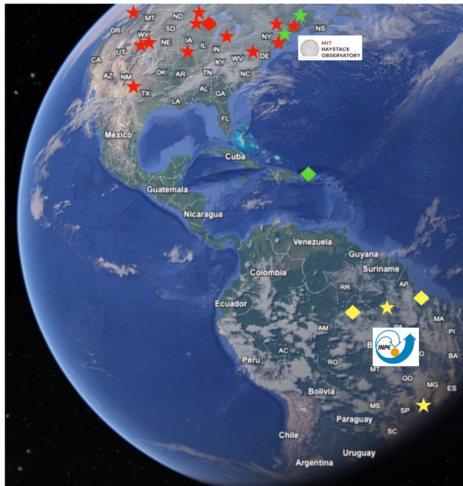
Figure 1: The location of all of CPI's instruments are shown in this figure. Stars indicate our instruments that are currently in operation. Diamonds indicate instruments that will be deployed in the future. Red and yellow indicate the location of our MagStar magnetometers and FPIs respectively. Green shows locations where we have several of our instruments operating in the same location.
