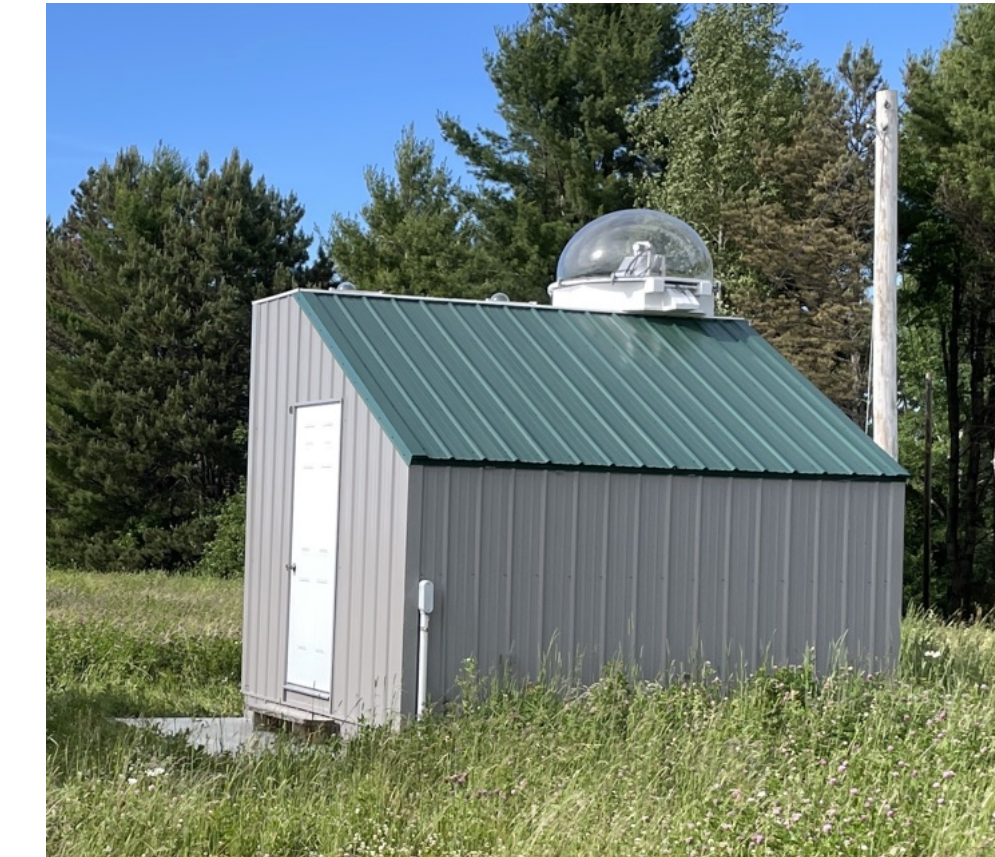
Figure 6: CPI provides the highest fidelity neutral wind measurements available to Space Weather operations (statistical wind uncertainties of < 0.5 m/s). Apart from our neutral wind measurements, we also obtain temperature measurements in all our locations. We show the FPI located at the Francis Malcom Science Center in Easton, MA.
