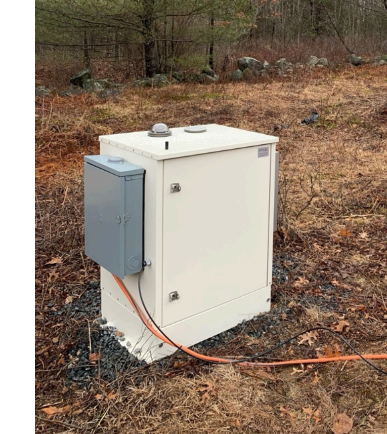
Figure 10: Our all-sky fisheye spectral imagers (ASIs) have a telecentric design that ensures all the chief rays are at normal incidence at the image plane, allowing the use of narrow bandpass interference filters (< 2nm) in the five-position filter wheel. We use the all-sky imagers to detect the position, morphology and evolution of the aurora and its characteristics, monitor for clouds, astronomical extinction measurements, meteor imaging and detection, aerosol and pollution monitoring and for security and surveillance.
