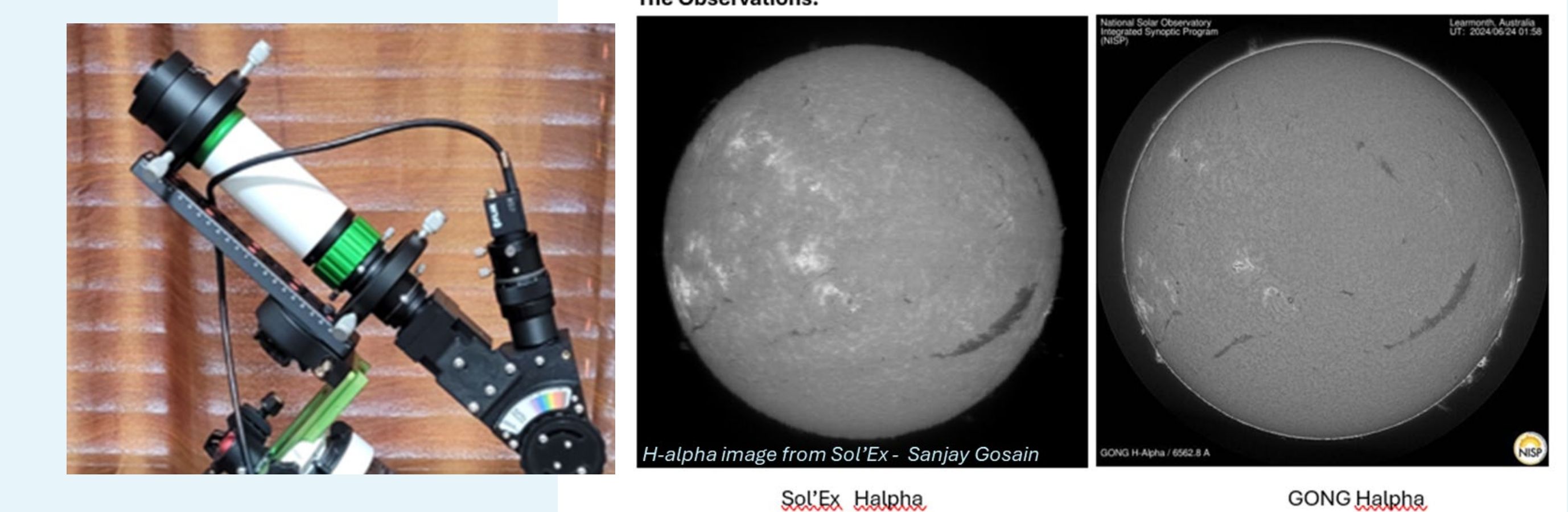
Figure 5: An early prototype of the spectroheliograph concept is shown on the left. The 3D printed Sol'Ex spectroheliograph (Buil 2021), popular among amateur astronomers was realized and tested for performance. The Sol'Ex has smaller optics (smaller grating and slit length) compared to our design, which is geared for higher resolution and employs larger optical components. The observations obtained from Sol'Ex are shown in the middle panel and a GONG H-alpha image is shown on the right panel for comparison.
