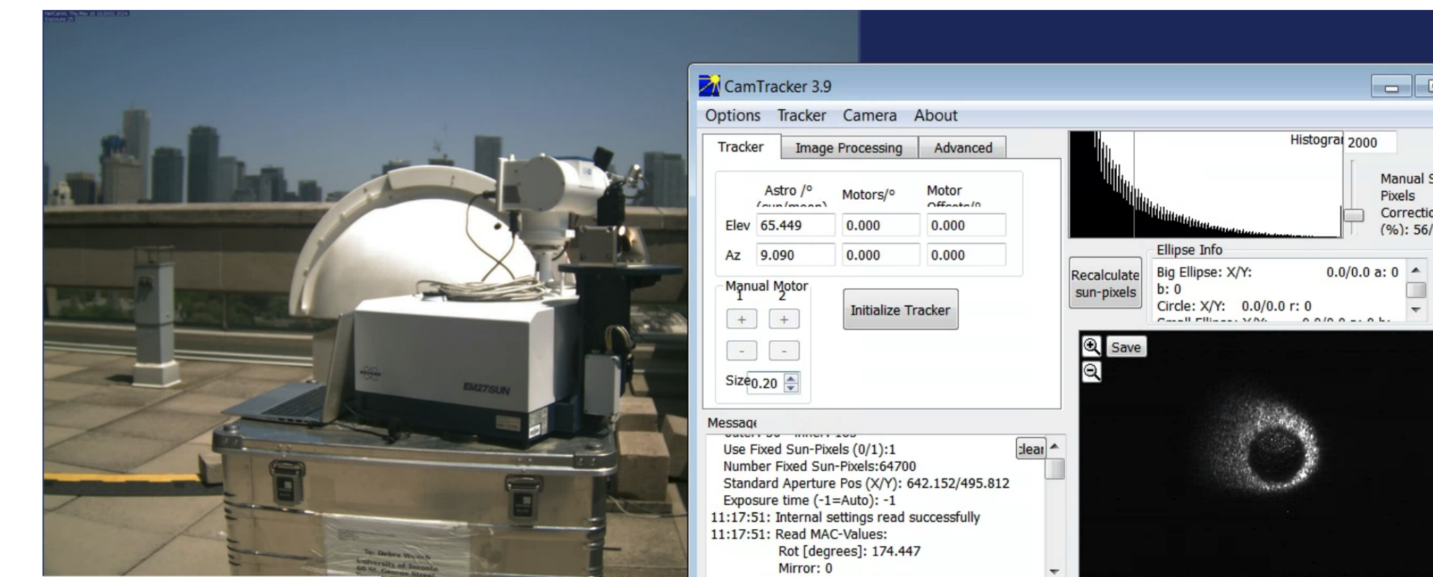
Fig. 6: Setup at the University of Toronto and camera image of the detector with CaF 2 lenses and 15 cm telescope, on 2024-05-16. A collocated EM27/SUN with standard tracker is also measuring.
