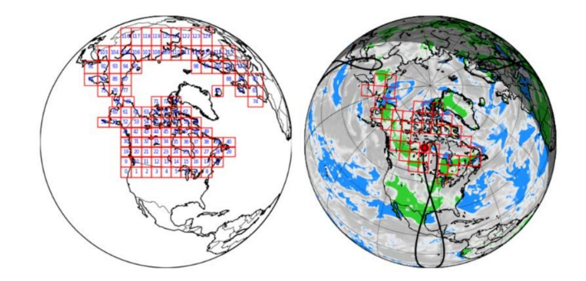
**Left:** Boxes show possible positions for 128x128 ~4x4 km<sup>2</sup> pixel field-ofview (FOV) from apogee at 95°W, accounting viewing angles. **Right:** Example of AOM IFTS FOV locations in 1 hour based on clouds (NASA MERRA-2 0.5°x0.67° cloud fractions >0.1), sunlight and view angles with satellite position (red circle) and orbit tracks (black line).
