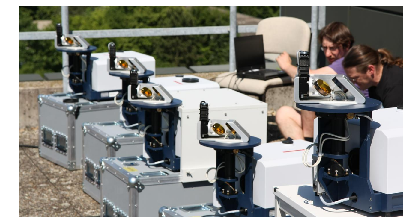
Calibration of EM27/Sun spectrometers; image from Frey et al. AMT, 2019.
