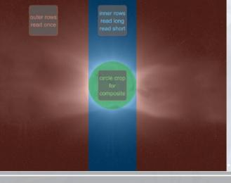
The SHDR scheme enables capture both the bright solar disk and faint corona in a single image. Columns corresponding to the solar disk use short exposures. while columns imaging the corona use longer exposures to enhance signal capture.
