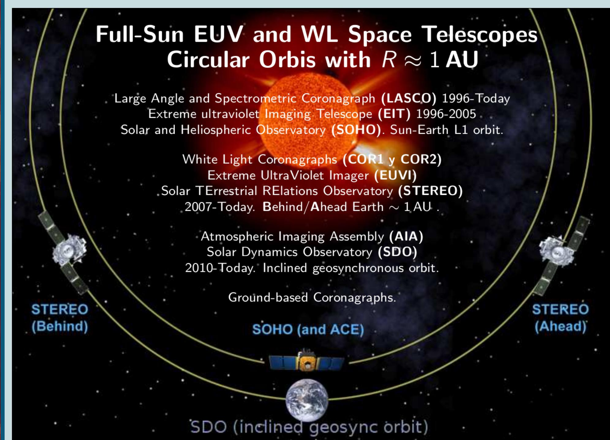
Using EUV images taken over 1/2 solar rotation ( $\approx 14$  days) with space telescopes (SOHO/EIT, STEREO/EUVI, SDO/AIA), SRT allows 3D reconstruction of the coronal emissivity in their various bands.
