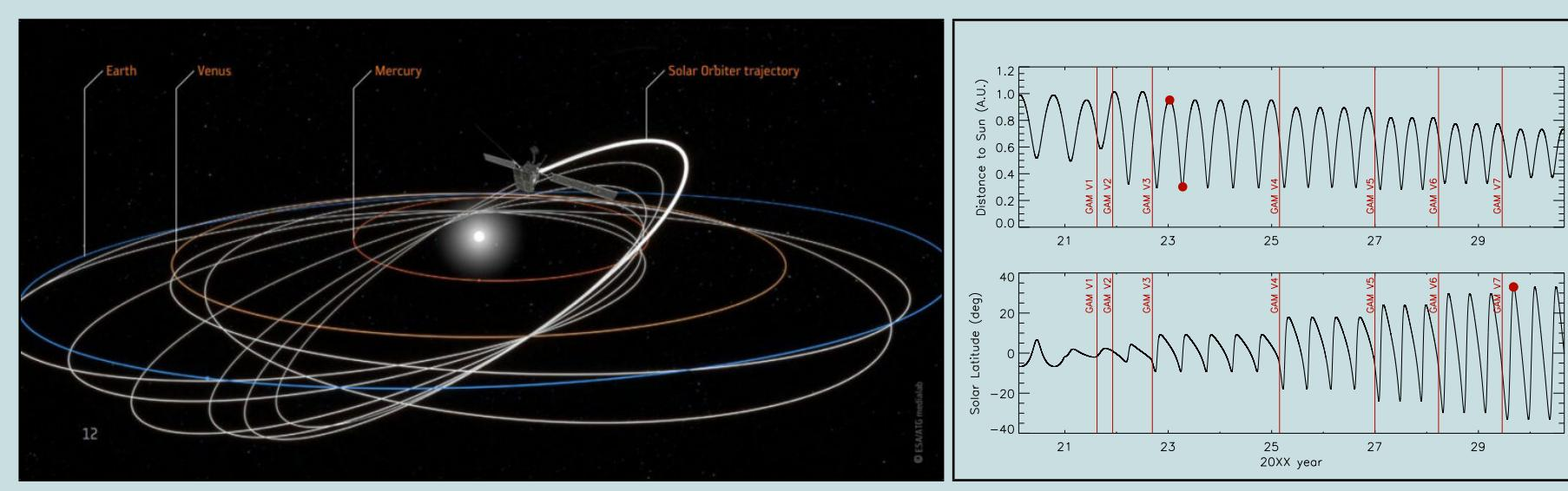
As SOLO flies the Metis FOV varies from  $\approx 5.8 \rightarrow 10.2$   $R_\odot$  at its maximum aphelion  $\approx 1$  au, down to  $\approx 1.7 \rightarrow 3.0$   $R_\odot$  at its minimum perihelion  $\approx 0.28$  au.
