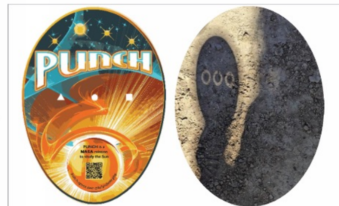
Fig. 1. Our 3-Hole-PUNCH Pinhole Projector (left) reveals the "ring of light" (right) during the October 2023 annular eclipse viewed from Chaco Canyon. The Projector is available in both English and Spanish.
